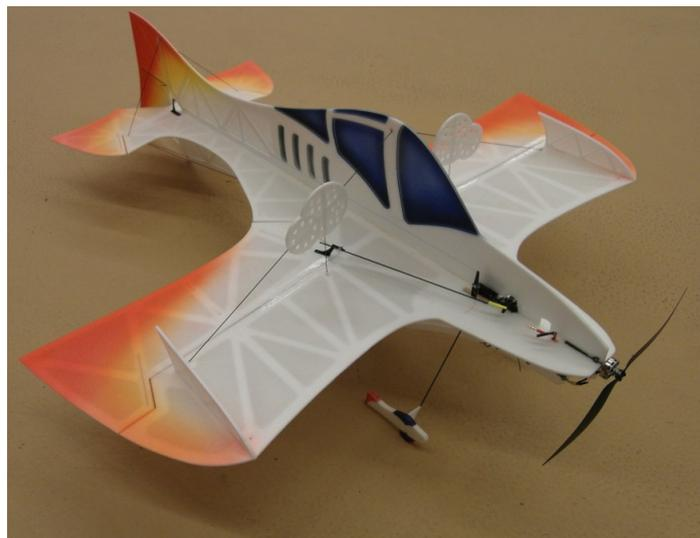
The production plane as shown in the picture is just a bit over 100 gram. The following equipment was used: JR-188 for ailerons, Dymond4.7 for Elevator and Rudder, Glavak 12gram motor, Glavak9 x 3.8 prop, YGE4, Hyperion 160mAh 2S, Spectrum AR6100
